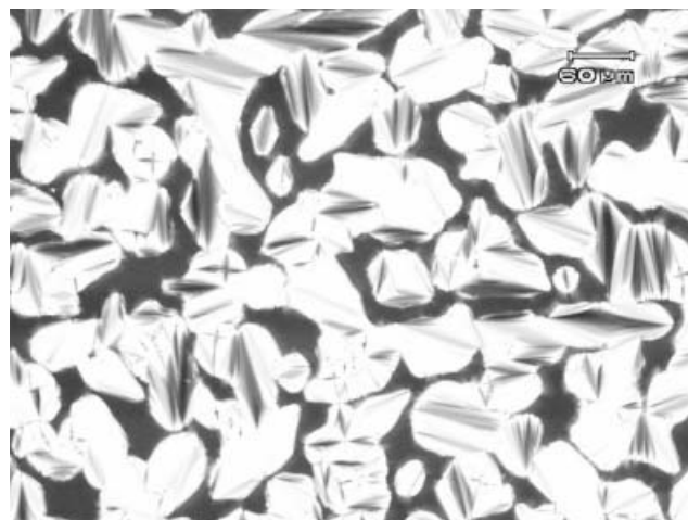
Figure 2. Optical microscopic texture showing the SmA phase (at 100°C) of compound 4 .
